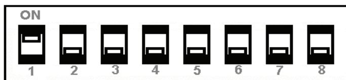
FIGURE 10: DIP SWITCH SETTINGS (SHOWING SETTING FOR IRDA)
